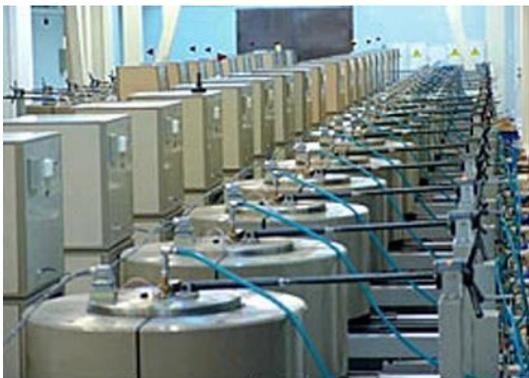
Figure 1: Cubic press at "Sundance Diamonds" for changing color of diamonds and BARS type presses at "AOTC" for growing diamonds.
