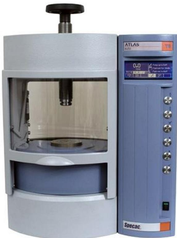
At left you are looking at an Atlas model Hydraulic Pellet Press made by the Specac™ company. This press is used to press materials into small pellets for preparation as study specimens for FT-IR, XRF and other lab testing.
