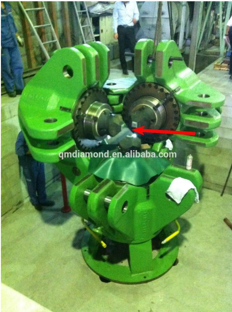
Again from the QMDiamond listings on alibaba dot com, we find a demonstration of a partially assembled diamond making press. The red arrow I have placed on the image to show exactly where the diamond making point is in this press. It requires a massive amount of pressure and heat to force carbon to crystallize.
