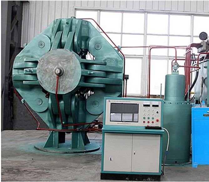
For educational purposes, I utilized these images from the QM Diamond company on alibaba dot com. Notice the size and shape of the press at left. It is designed to bring the extremely high pressure and high temperature required to duplicate the conditions approximately 150 km deep inside the earth. This is the area where carbon crystallizes and forms diamonds. It requires a machine press of this size and magnitude to accurately duplicate those conditions in a lab, as you see at left.
